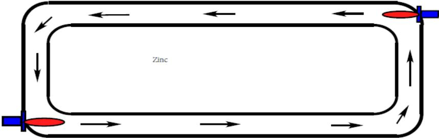
Figure 1 The pulse fire high-velocity type hot-dip galvanizing furnace layout
