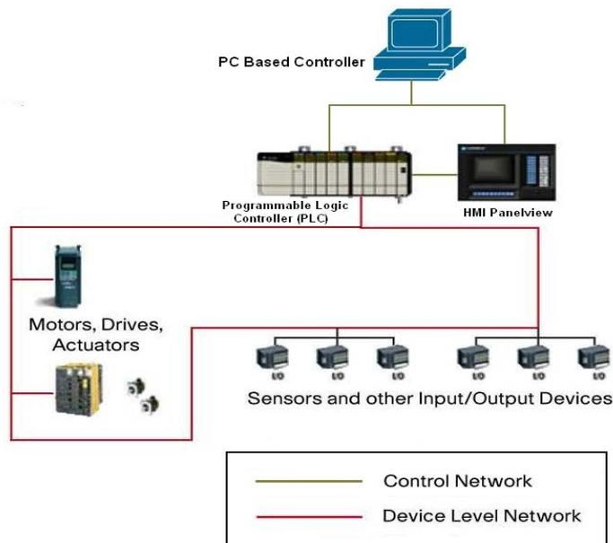
Figure 5 Hybrid PC/PLC control architecture
