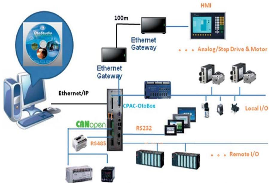
Figure 6 Computerized Programmable Automation Controller System
