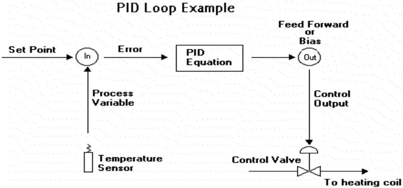
Figure 2 PID Loop Example
