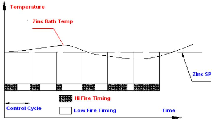
Figure 3 Typical High Fire, Low Fire and resultant furnace temperature
