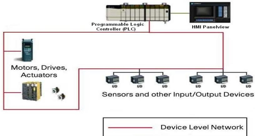
Figure 4, Typical PLC control architecture
