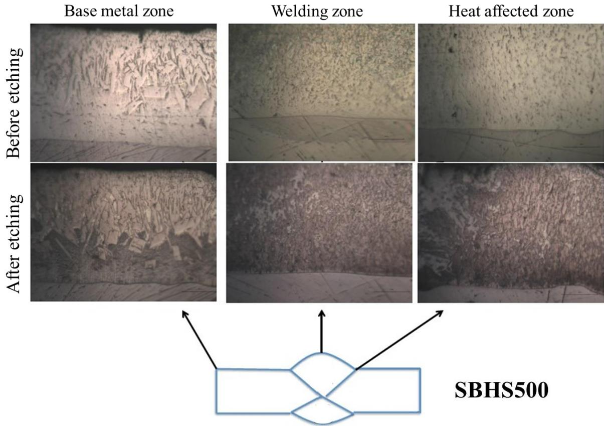
Fig. 6. Cross section of welded SBHS500 after HDG process before etching and after etching under OM.
