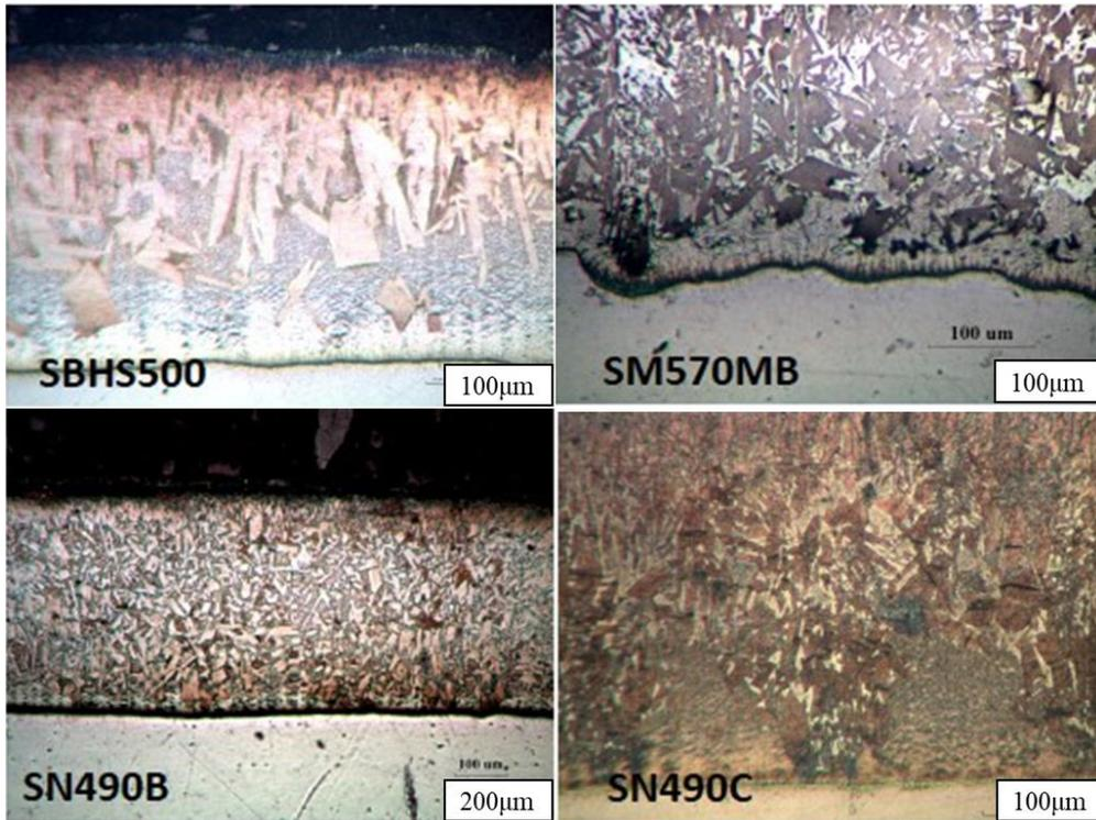
Fig. 1. Cross sections of SN490B, SN490C, SBHS500, and SM570MB under OM.
