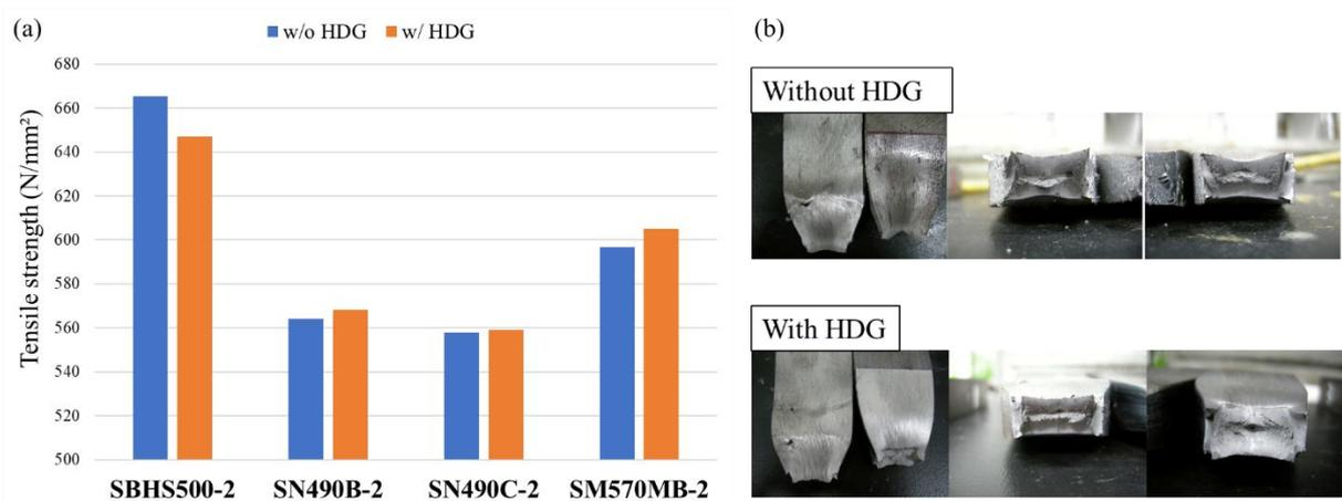
Fig. 7. (a) Tensile strength of different welded steels and (b) failure interface of SBHS500 with and without HDG.
