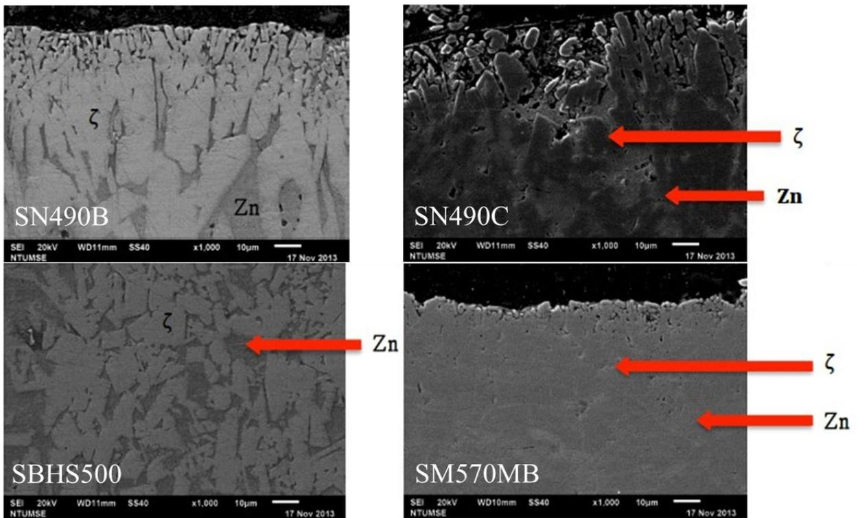
Fig. 2. Cross sections of SN490B, SN490C, SBHS500, and SM570MB under SEM.
