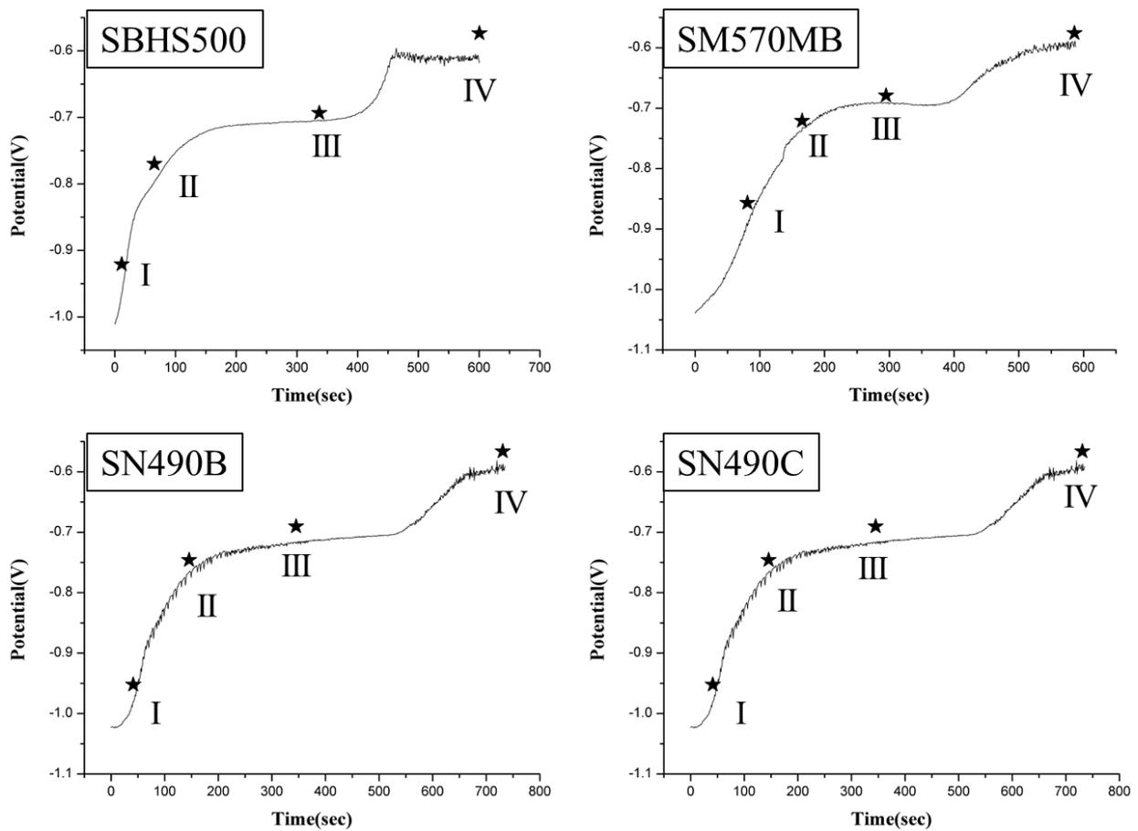
Fig. 3. OCP of SN490B, SN490C, SBHS500, and SM570MB in 7.5vol% HCl.
