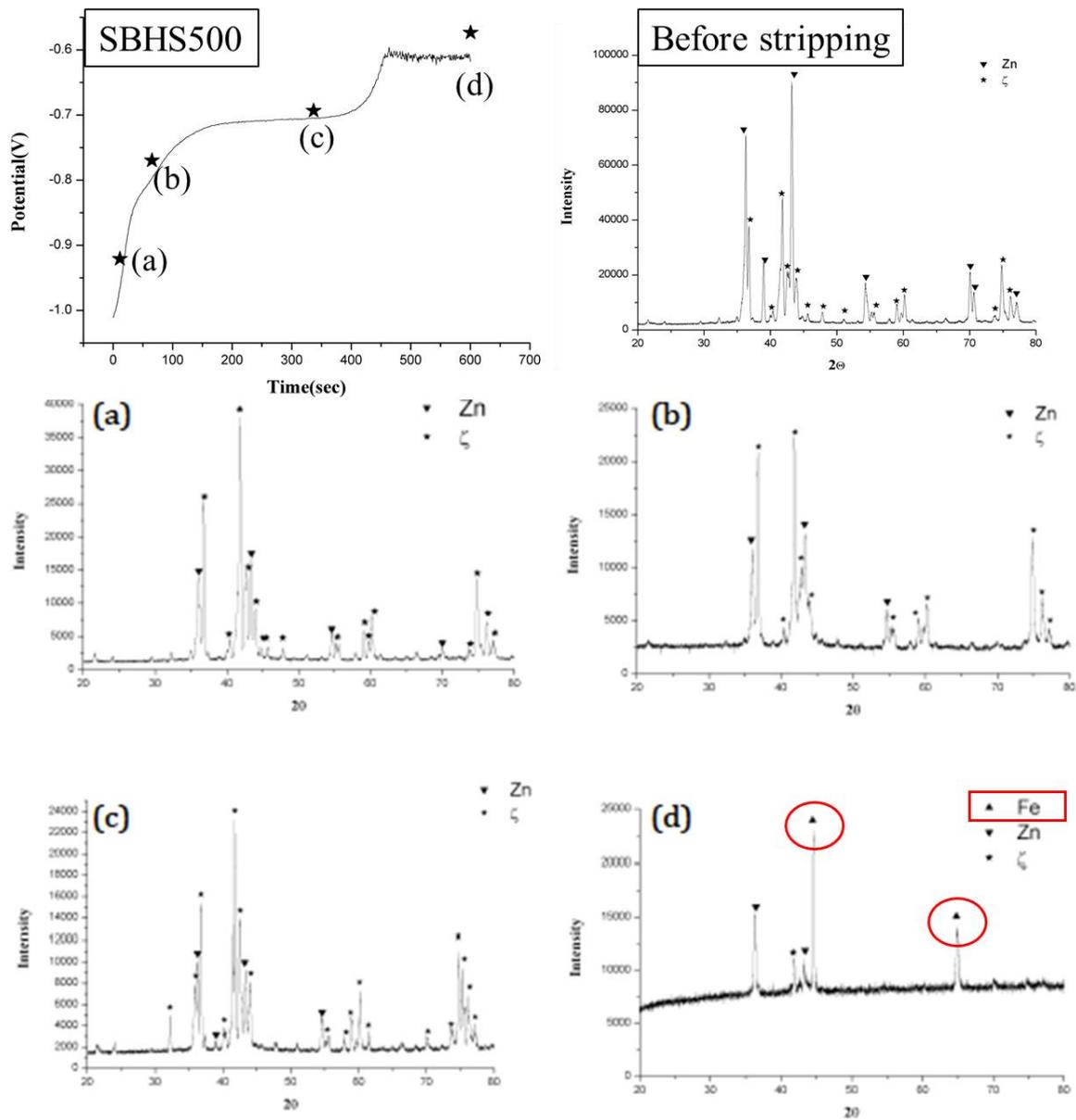
Fig. 5. XRD pattern prior to the chemical stripping of SBHS500, and the patterns from the start of the test at (a) 25 s, (b) 75 s, (c) 350 s, and (d) 650 s.
